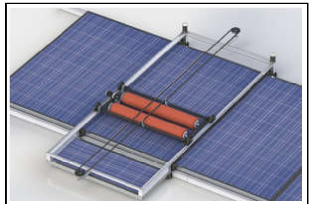
Fig.6 The inner frame attached to outer frame
