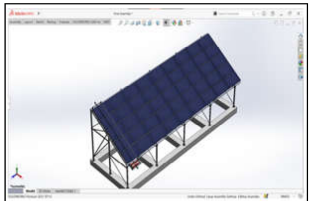
Fig.7 Automated cleaning system mounted on solar panel
