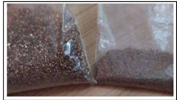
A. Before Sieving B. After Sieving Fig.2 Sieved Reinforcement Scrap Particles
